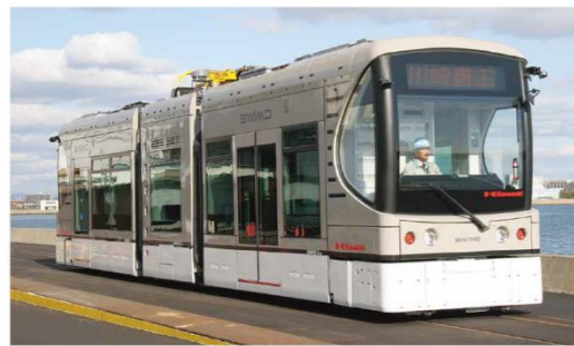
SWIMO low floor, battery-powered tram
