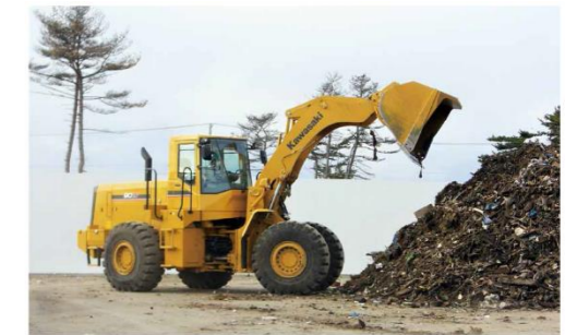
Wheel loader used for debris disposal and land leveling
