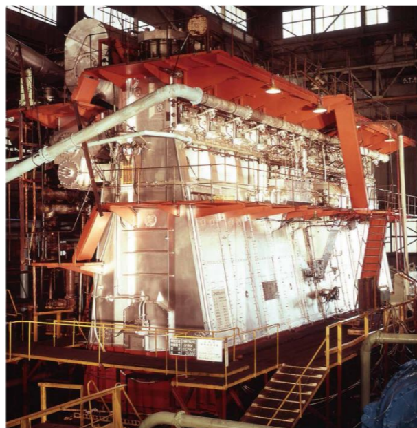
First model of Kawasaki-MAN K10Z93/170E diesel engine
