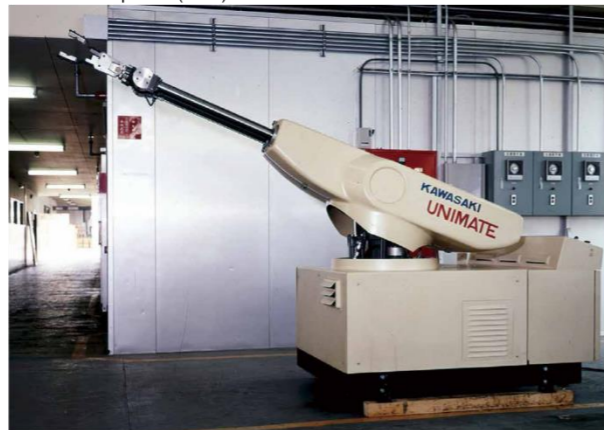
Kawasaki-Unimate 2000, the first Japan-made industrial robot completed in 1969
