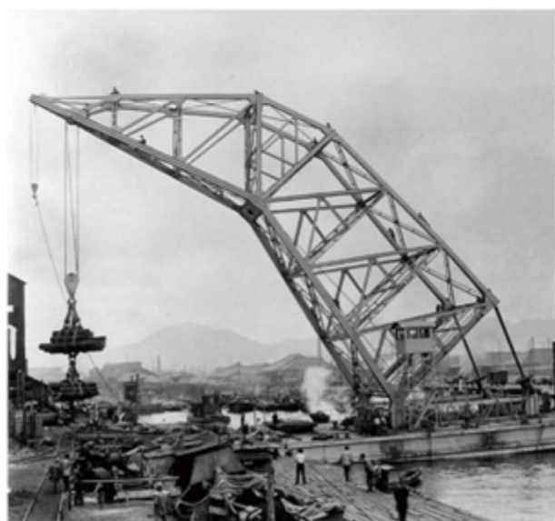
A 150 ton crane vessel and a railway pier at the far right (1908)
