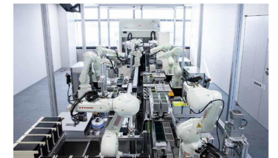
Automated robotic PCR testing system
