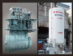
2S50ME-C GI and the fuel gas supply system. Gas
