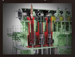
ME-GI has been designed based on 2-stroke diesel engine which has many records and high reliability.
