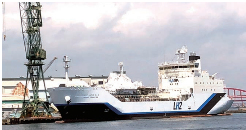
Fig. 8 Liquefied hydrogen carrier under outfitting (May 2020)
