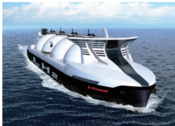
(c) Liquefied hydrogen carrier (160,000 m 3 capacity)
