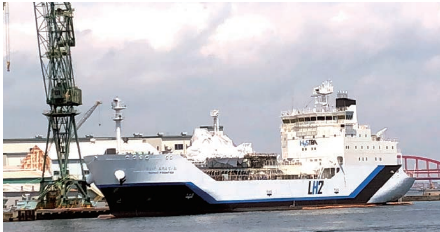
Fig. 8 Liquefied hydrogen carrier under outfitting (May 2020)
