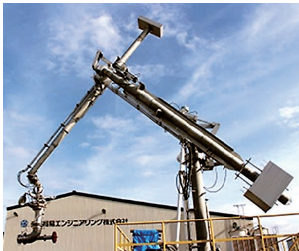
Fig. 8 Liquefied hydrogen loading arm systems for commercial use
