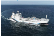
tank capacity : 1,250m 3
